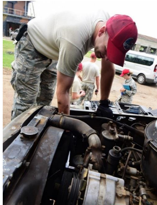
Staff Sgt. William Bennett, vehicle maintenance technician with the 201st RHS Engineers, tightens a belt during his completion of the preventive maintenance inspection of a water truck.
