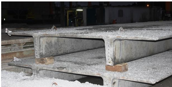
Completed double tee beams staged after curing and awaiting delivery to job site.
