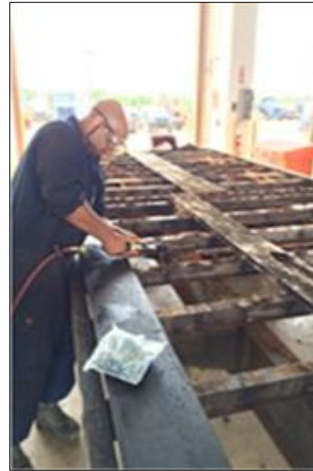
SrA Washington resurfacing a trailer deck.
