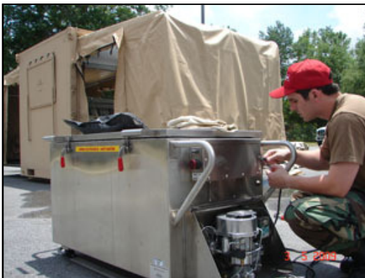
TSgt Joshua Crews helps operate the single pallet expeditionary kitchen (S.P.E.K.) during the 202nd RED HORSE field exercise at Camp Blanding. The S.P.E.K. is capable of feeding 550 people per meal, runs on a 2KW generator, and heats water using a "Babington Burner". Photo courtesy of SSgt Bill Nicholls.
