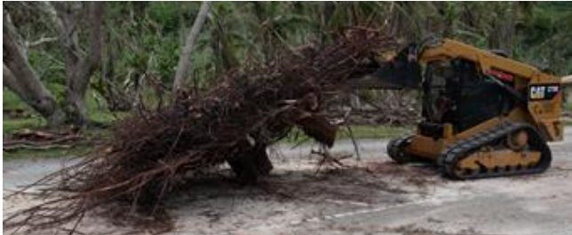
U.S. Air Force Master Sgt. William Harman, 36th Logistics Readiness Squadron operation superintendent, uses a compact track loader to lift tree roots.
