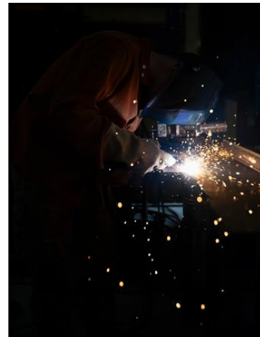
Senior Airman Collin Small, a structures specialist with the 157th CES, uses a plasma cutter to shape a steel plate. The week-long training prepared Airmen for rapid deployment operations by reinforcing core engineering tasks under austere, high-temperature conditions.
